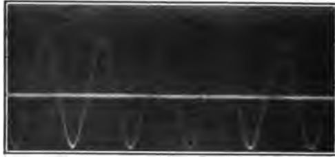
FIG. 104. The triple harmonic exciting current in the neutral of Y -connected transformers.
